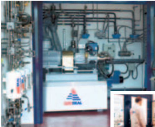
Computer controlled unmanned API 682 test facilities at AESSEAL plc UK Headquarters.
